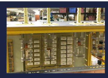
This large inductive reactor test system had to produce a programmable pulse of up to 50KV with a pulse rate of up to 250Hz. This system had to run continuously for may weeks.
